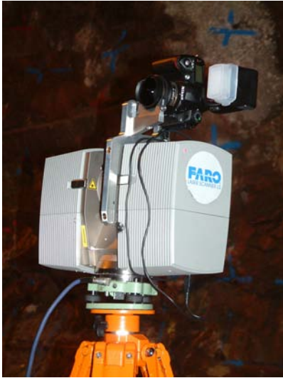
Laser scanner combined with digital camera
